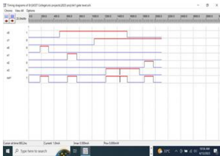
Fig. 8 : Timing diagram of Gate Level 4:1 Mux
